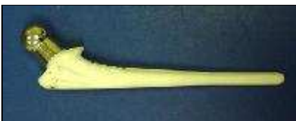
Metallic alloys. Composite stems combine the physical properties of alloys with those of other biomaterials. Note, ceramic or metal femoral heads are used on composite hip stems because composites have relatively poor wear properties.
