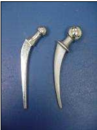
Metallic alloys. Stainless steel Charnley stem (left) and a cobalt-chromium Mueller (right).
