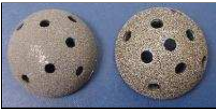
Metallic alloys. Tantalum (left) and titanium (right) fiber mesh acetabular cups.
